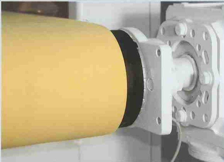
Rubberized conveyor drive drum
